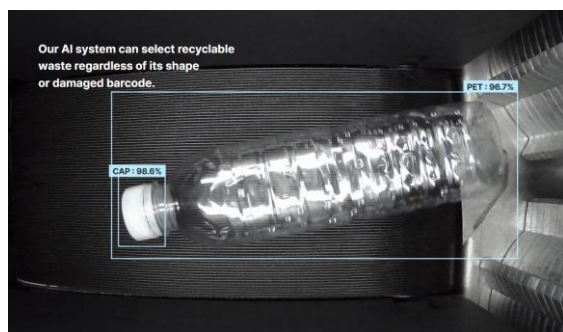
Figure 5. Application of Nephron's Image Sensing AI Technology
