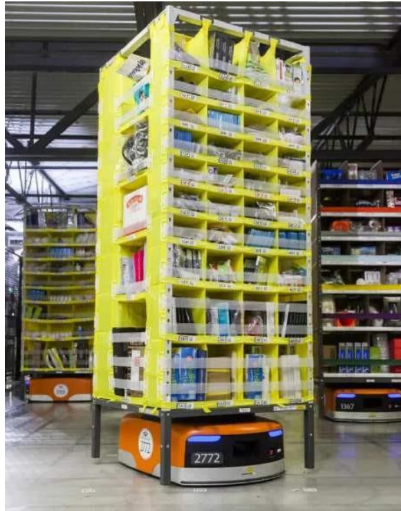
Figure 8: Robotized Amazon pods at an Amazon Robotics (AR) facility.
