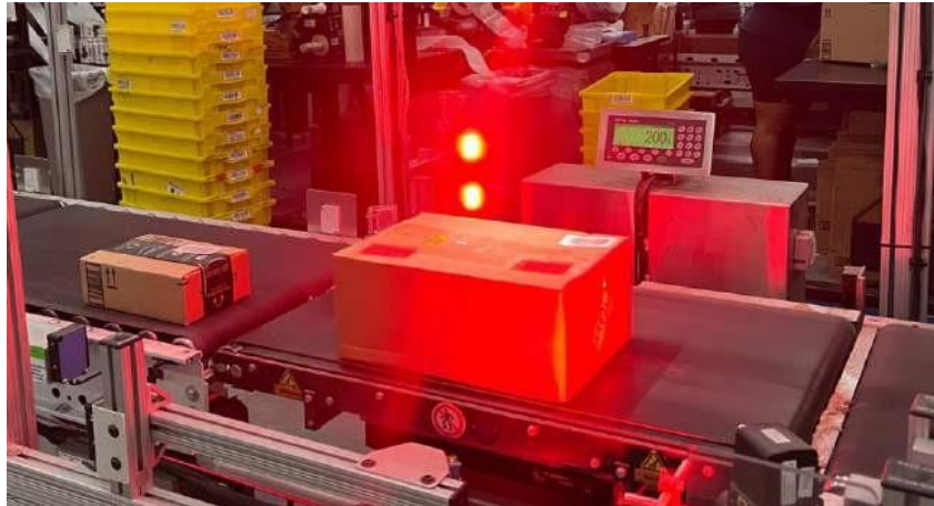
Figure 10: The SLAM (Scan, Label, Apply, Manifest) technology
