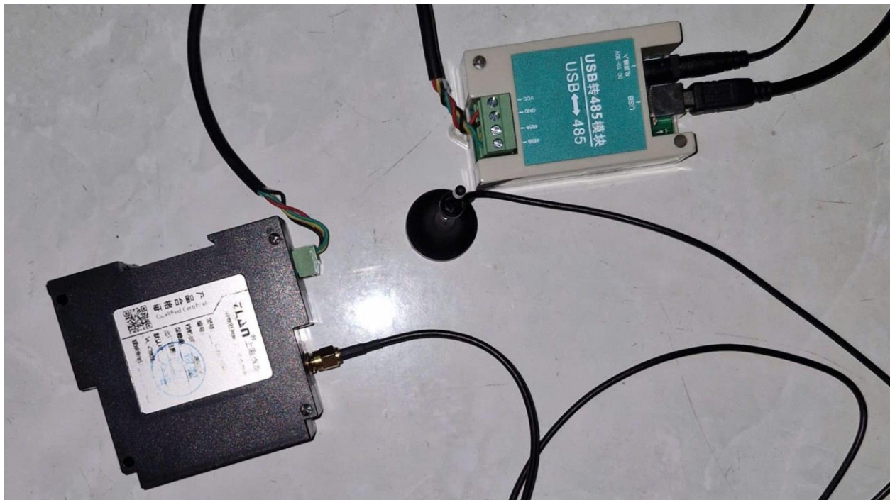
Figure 2: The RS485 to Wi-Fi Converter ZLAN7106M
