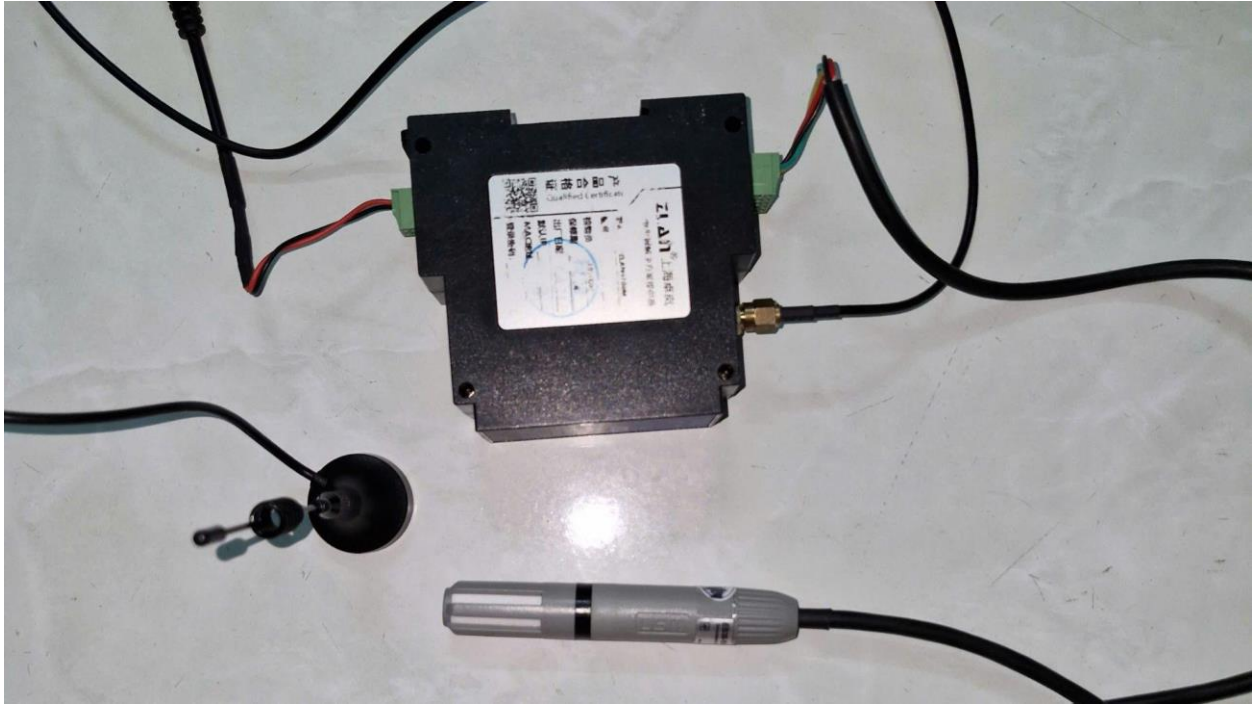
Figure 3: RS485 Modbus RTU Temperature and Humidity Sensor ES35-SW
